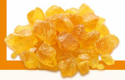
**Differentiating Amber and Copal:** Using the appropriate scratch sticks (or a fingernail) to test hardness, one should be able to tell quickly if the material is Amber or Copal. Amber has a hardness of 2-3 on Moh's scale while Copal registers around 1.5. Therefore, the Copal can be scratched with just a fingernail while the Ambar cannot.
